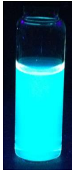
Figure S8. Photograph of green fluorescent Pt-NMQCs-Rec1-resilin nanobioconjugate dispersion under 365 nm UV light after storage at ambient temperature for almost a year.
