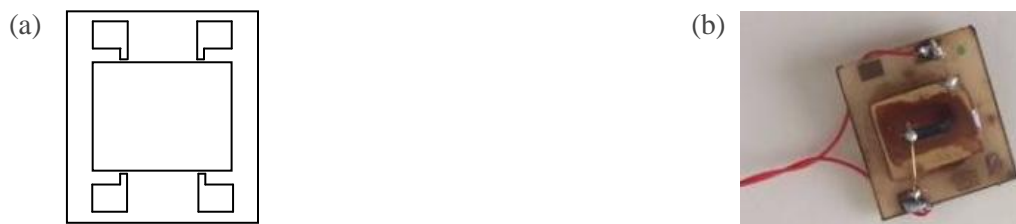
Figure S3: Description of the sensor assembly: a) Lay-out of the Electronic Mask (EM) and b) EM-Q-Cr-Au-TiO 2 -MIP Sensor
