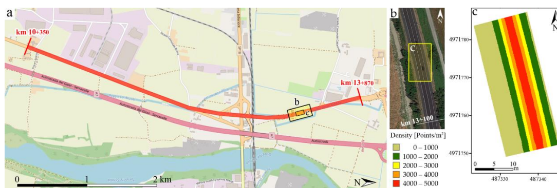
Figure 1. (a) Overview of the test site. (b) A picture of the section of a secondary suburban road. (c) Mobile laser scanner (MLS) cloud density map.
