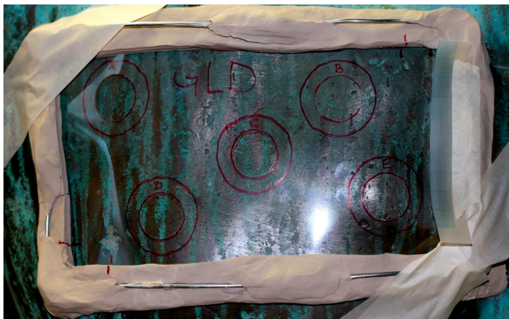
Figure 4. Frame used to reposition measurement instruments on a selected surface for monitoring purposes. A number of different areas are identified and labeled (A to D) for statistical reasons.
