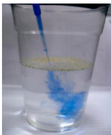
Figure 4. Water-penetrating or gateable property of the superhydrophobic sand floating on the free surface of water.
