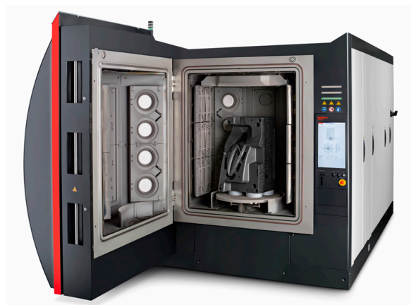
Figure 2. Medium-sized arc system equipped with circular arc evaporators, diameter 0.7 m, height 0.9 m, courtesy of Oerlikon Balzers.
