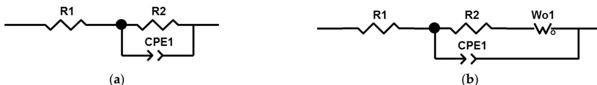
Figure 7. Equivalent circuits used for the electrochemical impedance spectroscopy (EIS) results fitting: (a) uncoated Ti and TZN substrates; (b) Ti+PEO and TZN+PEO coated samples.
