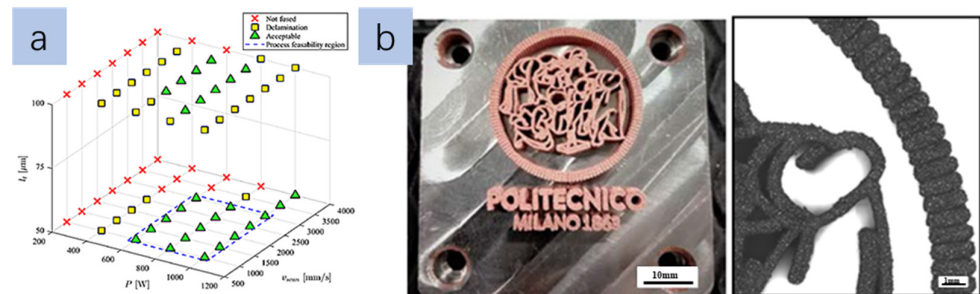
Figure 11. (a) Qualitative categorization of process outcome; (b) Final demonstrator produced by pure copper powder. Adapted from [42] Elsevier, 2018.
