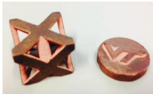
Figure 5. Complex-shaped copper made via binder jetting. Adapted from [19], MDPI, 2019.
