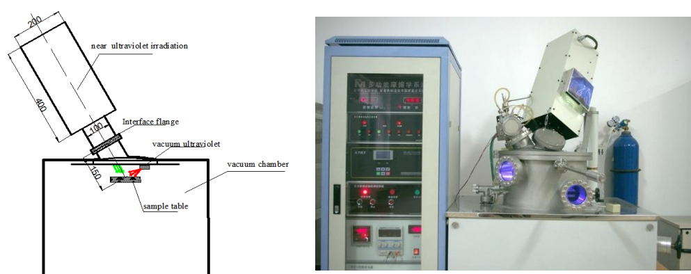
Figure 1. The schematic diagram of the UV radiation simulation device and MSTS-1 vacuum friction and wear tester integrated with UV radiation simulation device.
