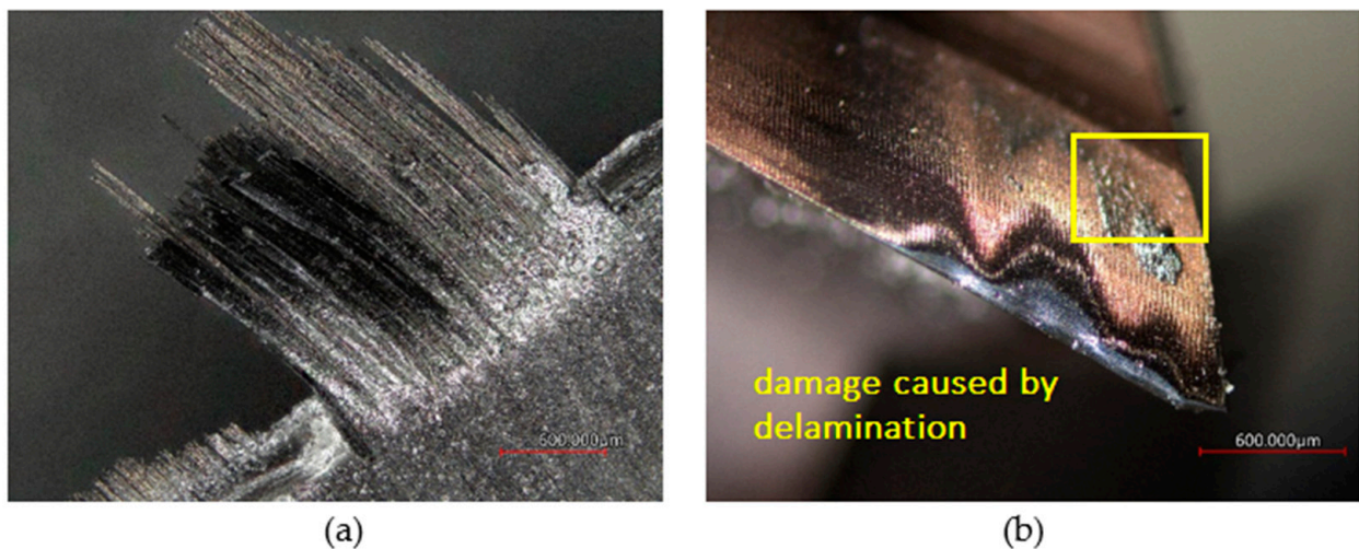
Figure 7. Capture after a tool tooth path of 15 \times 165 \text{ m} . (a) Laminate thickness 1 mm; (b) G550 milling tool.
