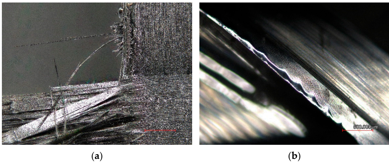
Figure 10. Capture after a tool tooth path of 15 \times 165 \text{ m} . (a) Laminate thickness 3 mm; (b) A100 milling tool.
