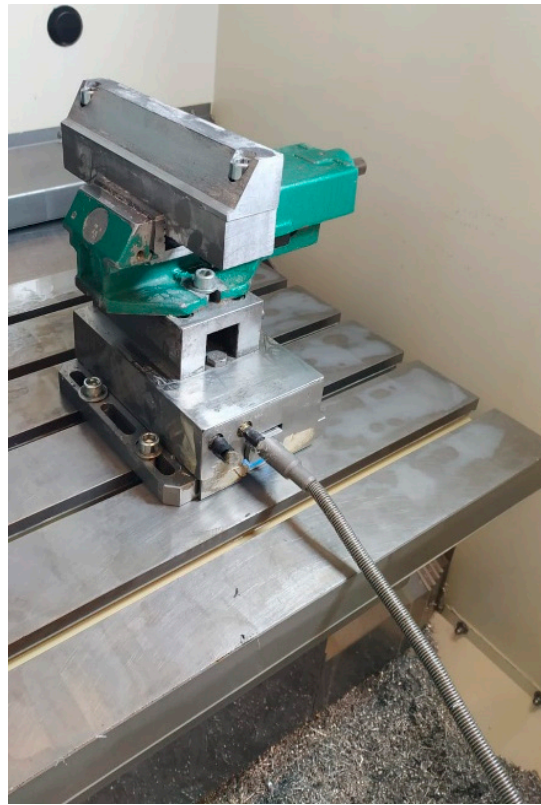
Figure 3. Fixture for mounting CFRP sample on the experimental device—piezoelectric dynamometer KISTLER 9265 B.
