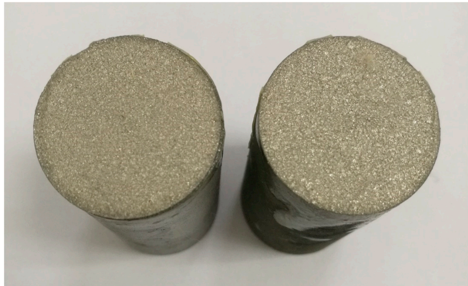
Figure 9. Macroscopic morphology of the fracture section of the BS test specimen.
