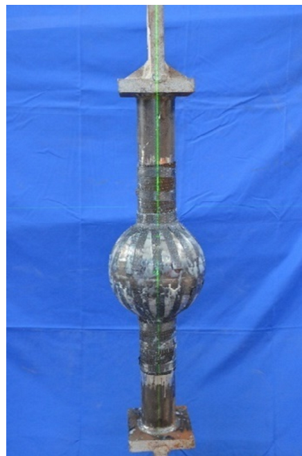
Figure 9. Specimen bonded with CFRP.
