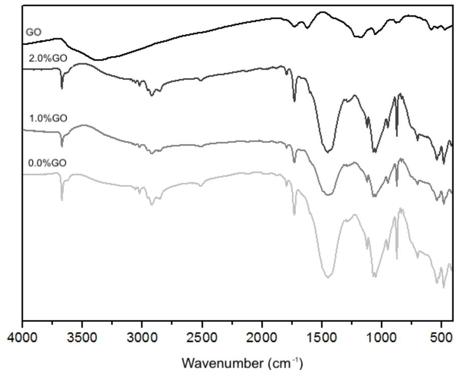
**Figure 4.** FTIR spectra of GO and wall latex paints with 0.0% of graphene oxide (GO), with 1.0% of GO and 2.0% of GO incorporation.
