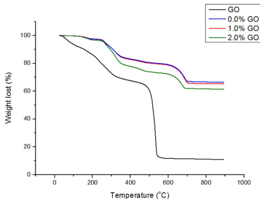
**Figure 5.** Thermograms of thermal analysis results for graphene oxide, wall latex paint without graphene oxide (GO), with GO 1.0%, and with GO 2.0% incorporation.
