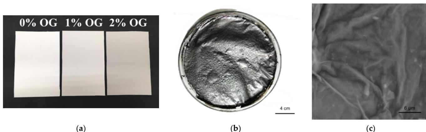
**Figure 1.** (a) Digital image of the coatings on a polycarbonate surface, (b) digital image of graphene oxide (GO) film, (c) SEM micrograph of GO film.
