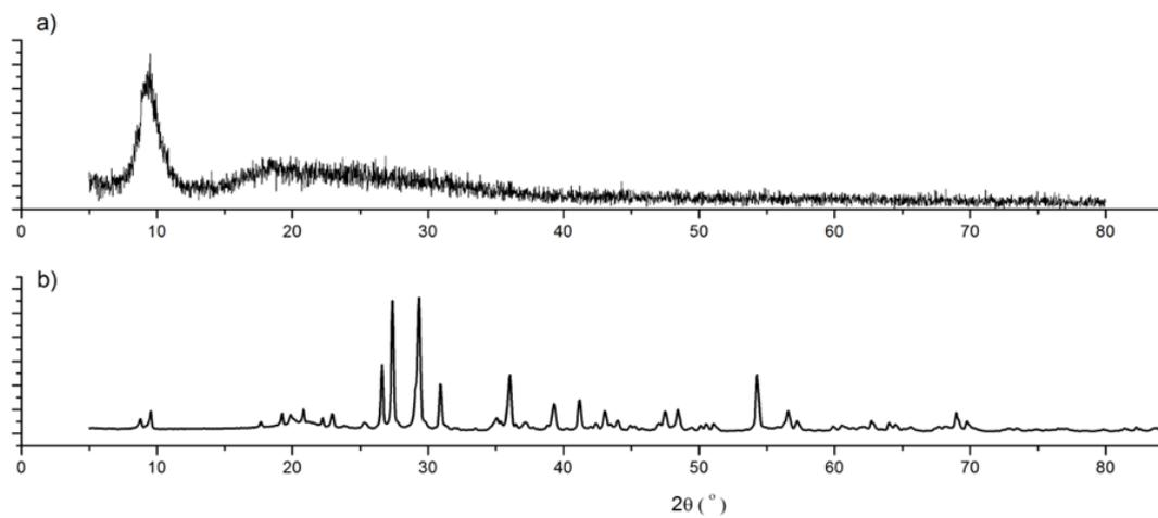
**Figure 3.** (a) XRD diffractogram of graphene oxide (GO) and of (b) wall latex paint with 2.0% of graphene oxide (GO) incorporation.
