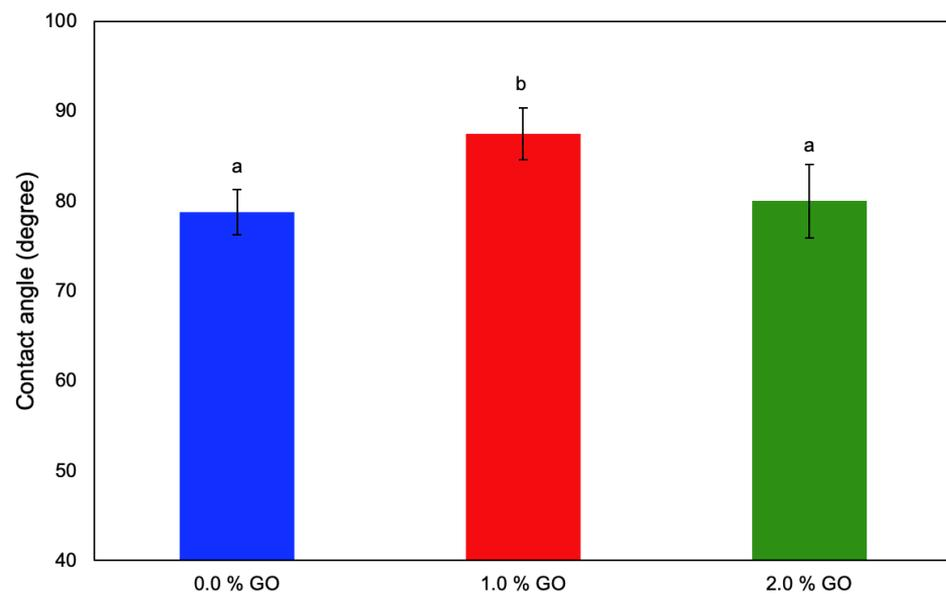
**Figure 6.** Static contact angles of water drop on the surface of wall latex paint without graphene oxide (GO), with 1.0% of GO, and with 2.0% of GO incorporation. The results marked with letter “a” do not differ statistically by Tukey test at a 5% of significance level.
