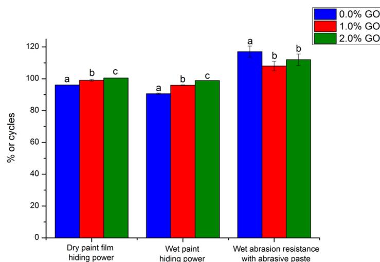
**Figure 7.** Evaluation results of wall latex matt paints developed with and without the incorporation of graphene oxide (GO). The results marked with the same letter do not differ statistically by Tukey test at a 5% of significance level.
