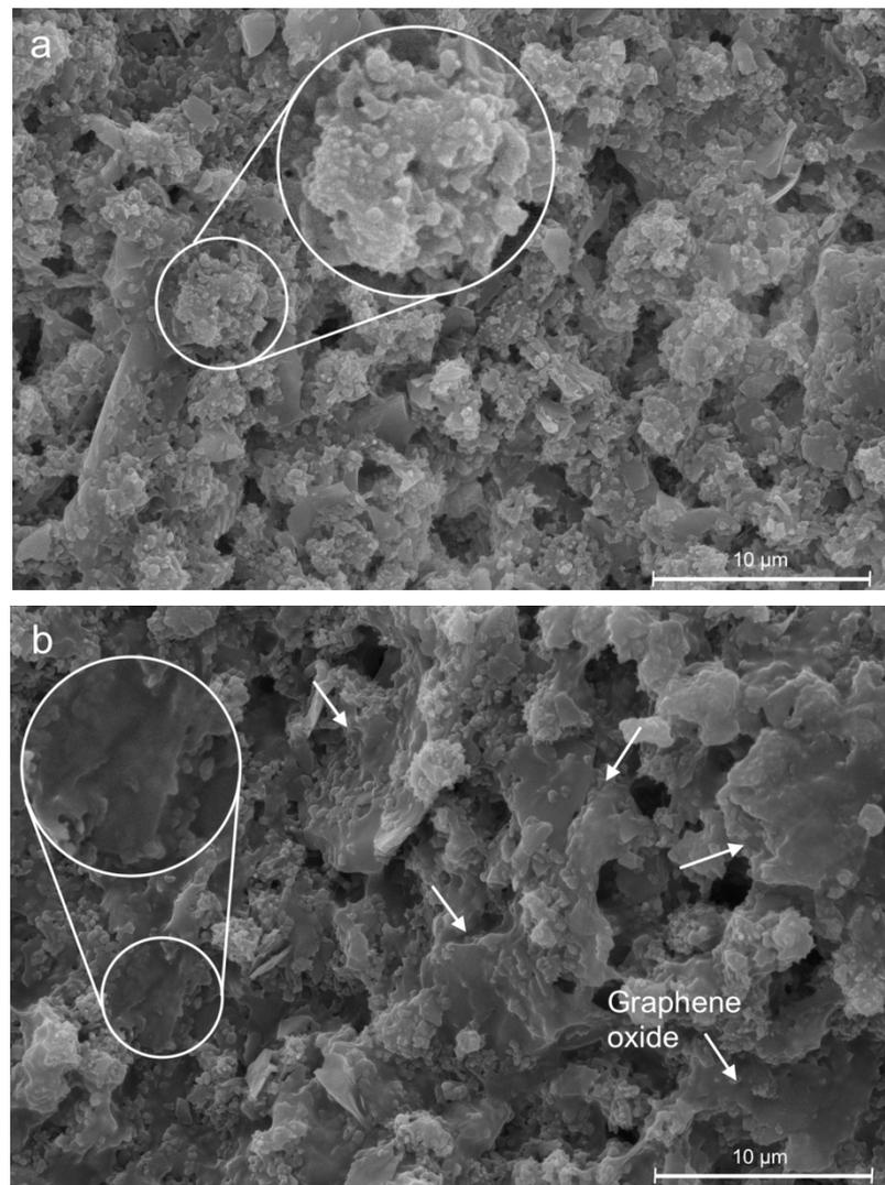
**Figure 2.** (a) SEM micrograph of the coating without the addition of graphene oxide (GO) and (b) SEM micrograph of the coating with 2.0% of GO incorporation.
