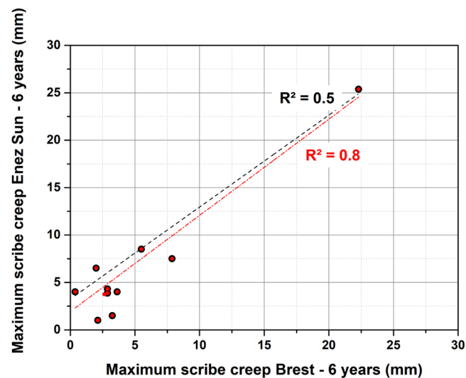
Figure 9. Linear regression plot between the maximum scribe creep before coating removal (M1) for Brest and Enez Sun. The red plot is the linear regression plot, with S7 excluded.
