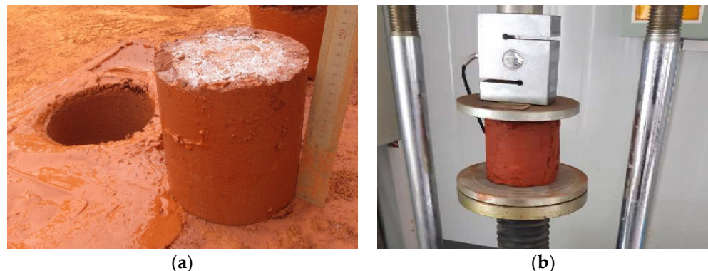
Figure 9. Site coring and testing of Bayer red mud Subgrade. (a) is field coring sample, (b) is unconfined compressive strength test of core sample.
