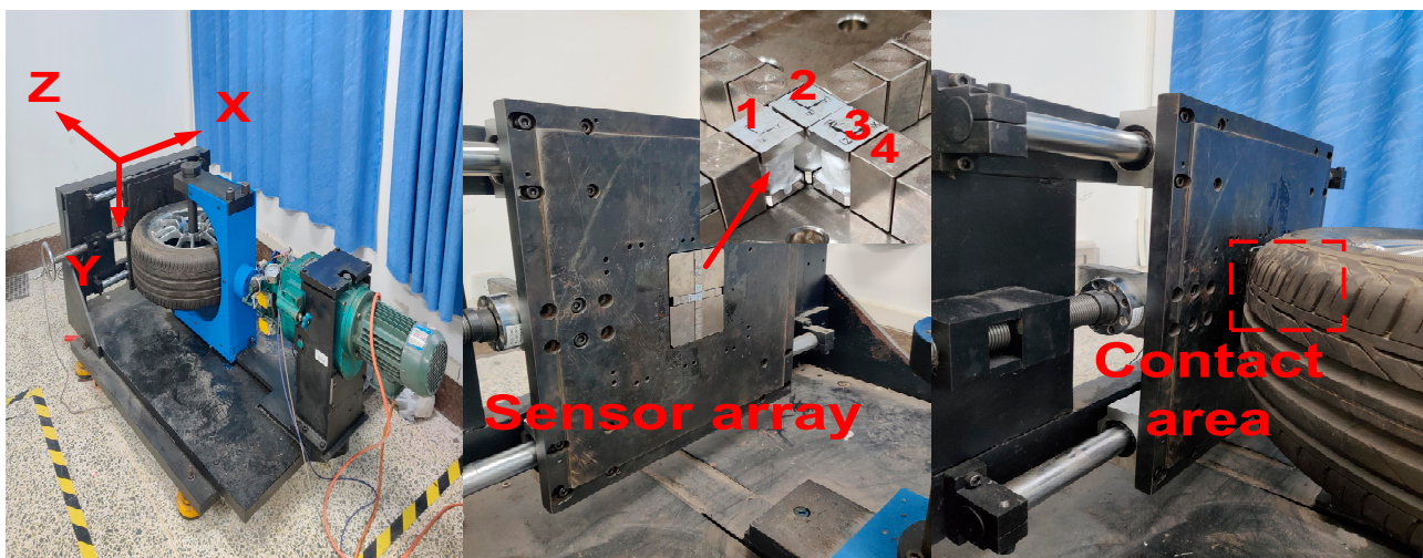
Figure 8. Simulated tire–pavement contact load test platform.
