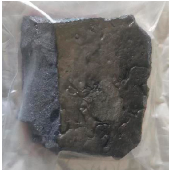
Figure 6. \text{Mg}_{30}\text{Zn}_{30}\text{Sn}_{30}\text{Sr}_5\text{Bi}_5 (at%) alloy block ( 40\text{ mm} \times 40\text{ mm} \times 20\text{ mm} ).
