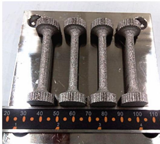
**Figure 10.** Tensile test sample manufactured by SLM.
