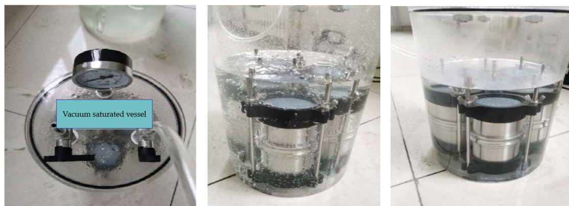
(a) Vacuum saturated containers (b) During vacuum saturation (c) End of vacuum saturation
