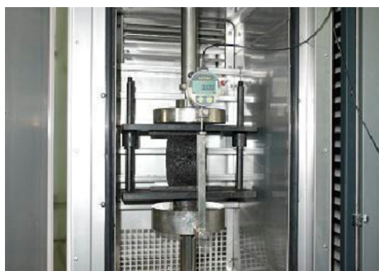
Figure 7. Low temperature freeze–thaw splitting test.
