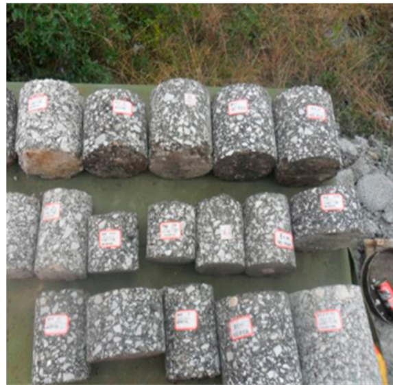
Figure 4. Samples of different CRM structure test sections.
