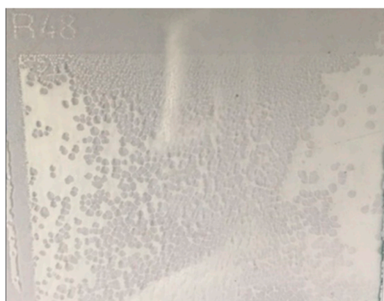
Figure S4. Example of gravure printed PVDF on PET-ITO substrate pre-treated by Corona at a power of 50 W.
