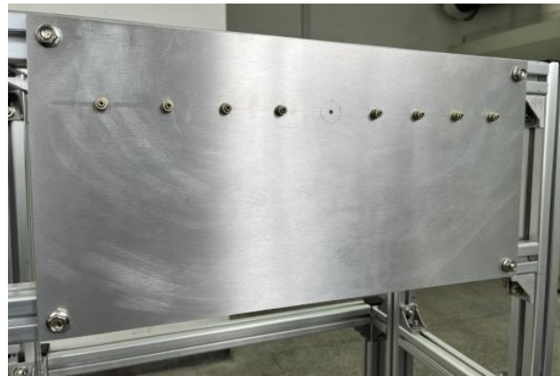
Figure 16. Specimen installed hi-lok nuts.
