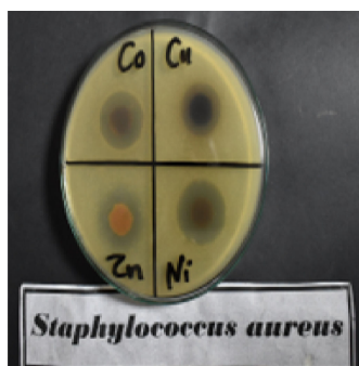
Cotton modified of Co(II), Ni(II), Cu(II), and Zn(II) complexes activity against S. aureus . (technique 2)
