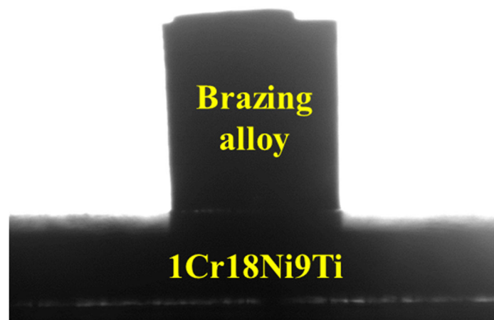
Figure S1. Side view of the base substrate and brazing alloy.
