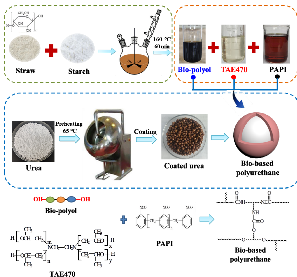
Scheme 2. Schematic diagram for the fabrication process and chemistry origin of bio-based polyurethane-coated urea.
