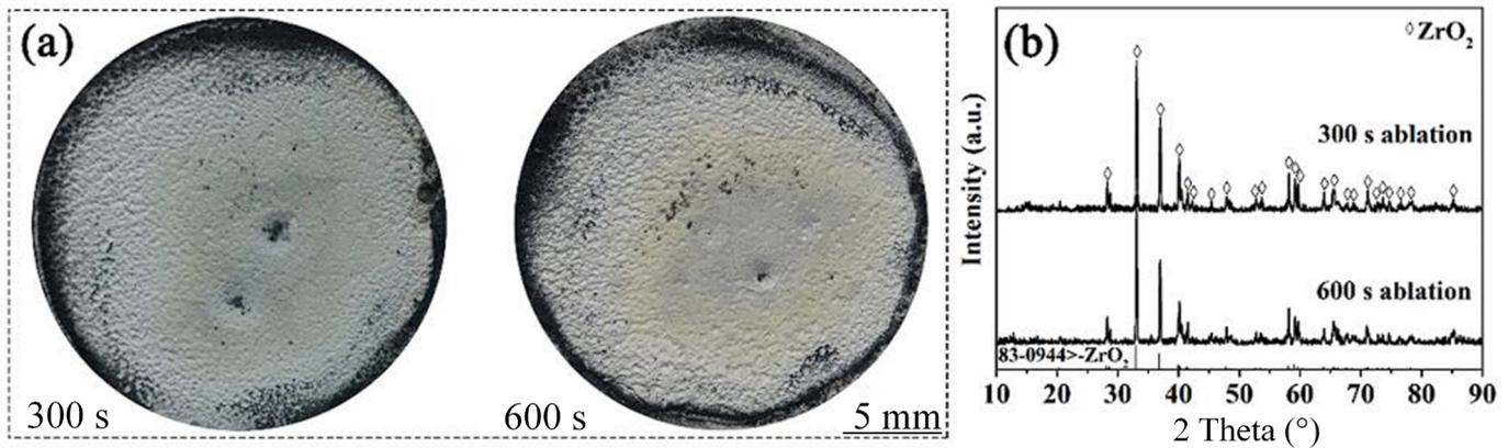
**Figure 5.** Ablative properties of ZrC–SiC coatings. (a) Appearance and (b) XRD properties of coatings ablated at various times. Reprinted/adapted with permission from Ref. [121]. Copyright 2022, Elsevier.
