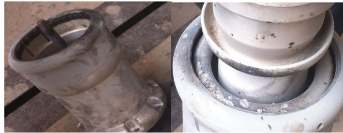
Figure 6. Contact photos of the test circuit breaker.
