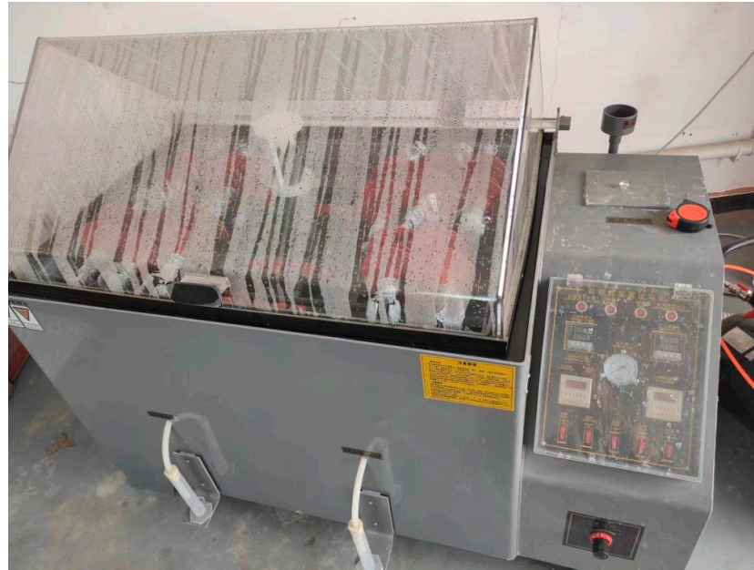
Figure 5. Salt spray ageing test platform.
