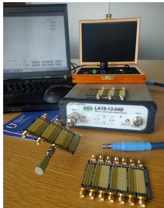
Figure A1. The experimental setup of the measurement test bench with LA19-1304B VNA.
