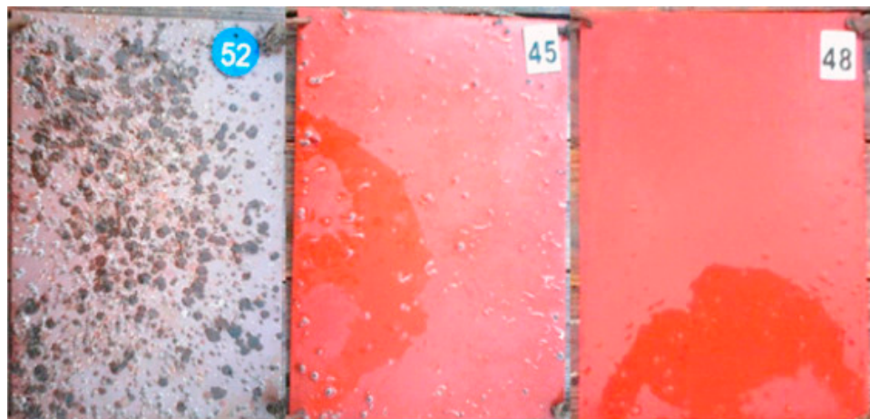
Figure 6. Images of marine antifouling coatings comprising stainless steel plates coating paint after immersion in the South China Sea (N 22°33', E 114°32') for a month. (No. 52) Control plat; (No. 45) Hydrophobic coating; and (No. 48) Hydrophilic coating [93]. Figure reproduced with permission from Progress in Organic Coatings (Elsevier).
