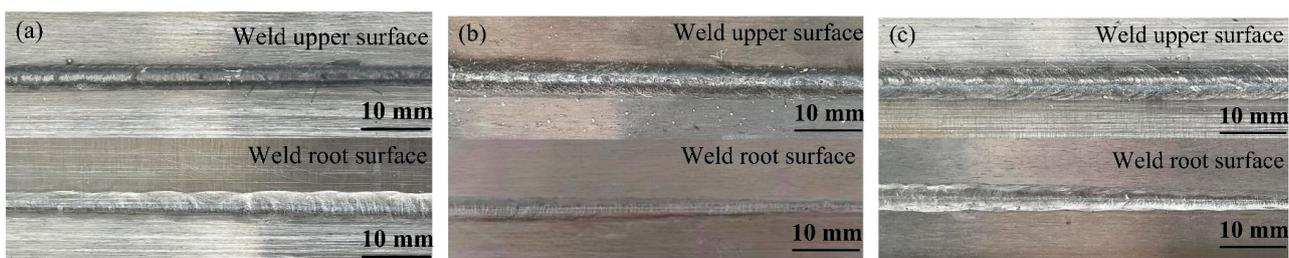
**Figure 6.** Macroscopic morphology of the weld under varying laser powers: (a) 1.50 kW; (b) 1.75 kW; (c) 2.00 kW.
