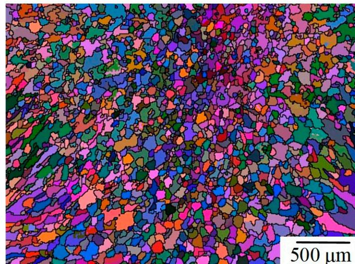
Figure 9. Euler diagram of the WJ when the laser power was 1.75 kW.
