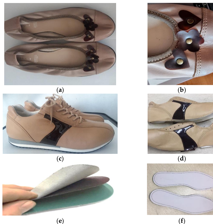
Figure 7. Incorporation of casein films into shoes: (a) and (b) G40/T5; (c) and (d) G60/T5; (e) and (f) G60/T10, middle layer.
