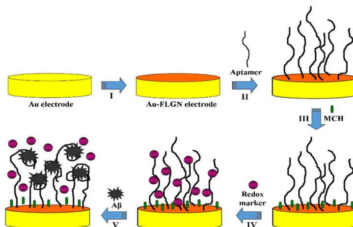
**Figure 2.** The scheme of fabrication of the aptasensor and A $\beta$  detection: I—electrode position of FLGN, II—aptamer immobilization, III—MCH immobilization, IV—A $\beta$  incubation. Adapted with permission from Ref. [114].
