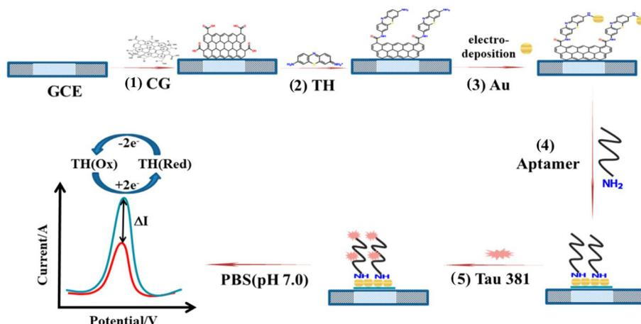
**Figure 4.** Schematic representation of tau-381 detection with the aptamer-based biosensor: (1) Doped CG on a GCE surface. (2) The incubation with Thi. (3) Electrodeposition and reduction of HAuCl<sub>4</sub>·3H<sub>2</sub>O to AuNPs. (4) Immobilization of aptamer. (5) The detection of tau-381 levels in HS by using DPV technique. Reprinted with permission from Ref. [136].
