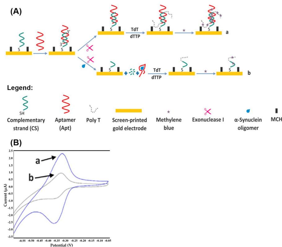
**Figure 1.** (A) Schematic illustration of voltammetric detection of  $\alpha$ -syn oligomers. (B) CV curves obtained for the sensing platform (a) in the absence and (b) in the presence of  $\alpha$ -syn oligomers. Measurements were carried out in PBS solution, scanning from  $-0.6$  V to  $-0.05$  V at a scan rate of  $100$  mV/s. Reprinted with permission from Ref. [102].
