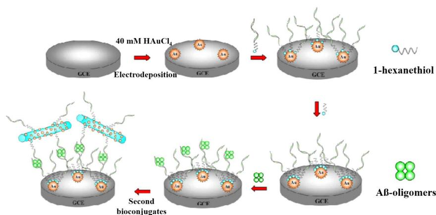
**Figure 3.** Schematic illustration of the fabrication of the aptasensor for A $\beta$ O detection. Reprinted with permission from Ref. [116].
