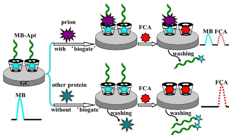
**Figure 6.** Schematic illustration of the voltammetric aptasensor for prion protein detection. Reprinted with permission from Ref. [142].
