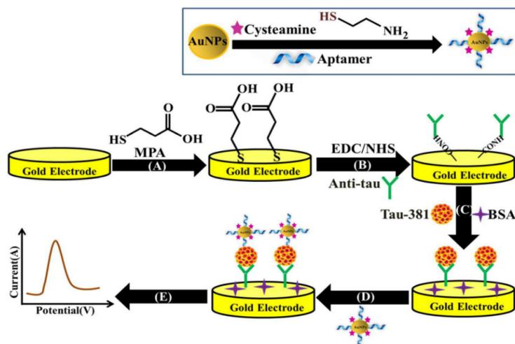
**Figure 5.** Preparation of Ab-Apt sandwich biosensor for detection of tau-381 protein: (A) Self-assembly of MPA at AuE. (B) EDC/NHS activation and anti-tau antibody immobilization. (C) Free sites blocked with BSA followed by immunoreaction with tau-381. (D) Affinity interaction the aptamer-Au-Cys bioconjugate. (E) Detection of tau-381 levels by using DPV. Reprinted with permission from Ref. [137].
