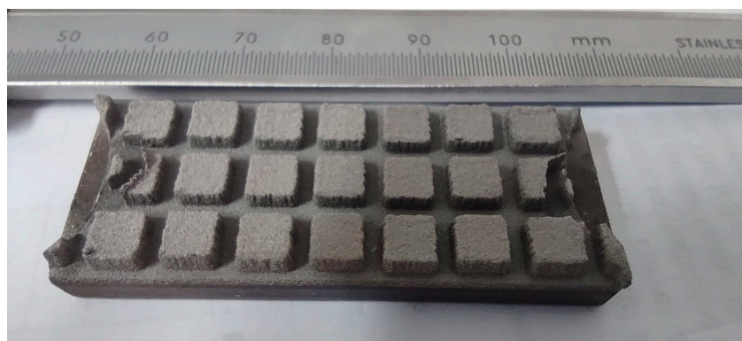
Figure 8. CSAM-ed Ti on stainless steel using masking strategy. Unit: mm.
