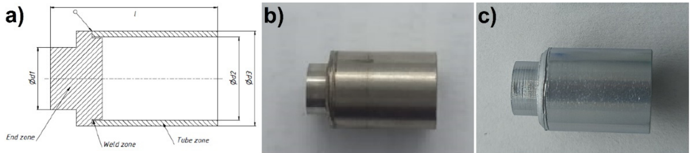
Figure 1. The schematic drawing of an RUW specimen (a). Appearance of (b) uncoated and (c) Cr-coated RUW E110 alloy specimens before hydrogenation tests.
