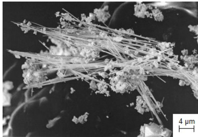
Figure 20. SEM image of TaO obtained by electrolysis of the CsCl-K 3 TaOF 6 (2.5 wt.%) melt at 1023 K and a current density of 0.15 A cm -2 .
