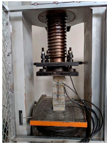
Figure 2. WHY-2000 electro-hydraulic servo pressure testing machine.
