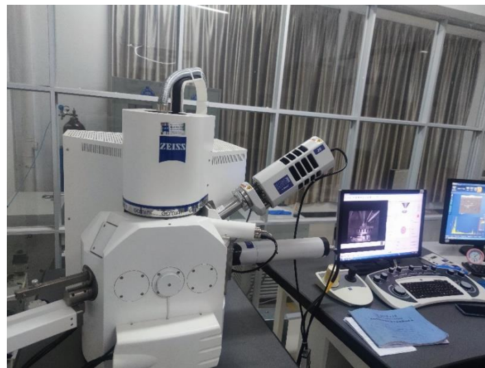
Figure 2. Electron microscope (ZEISS Sigma) with spectrometer.
