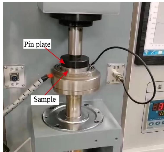
Figure 3. MMW-1A friction and wear testing machine.
