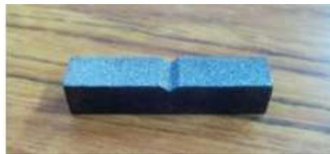
**Figure 3.** A sample for Charpy tests.
