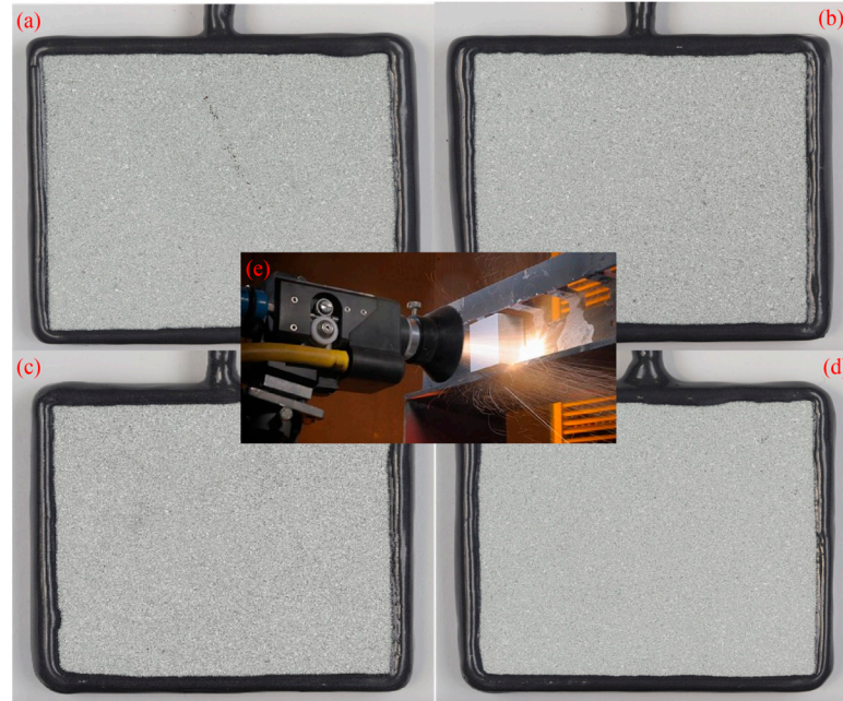
Figure 1. Schematic diagram of arc spraying and samples (a) 0.15 mm Zn, (b) 0.30 mm Zn, (c) 0.15 mm Zn/Al, (d) 0.30 mm Zn/Al, (e) Spray diagram.
