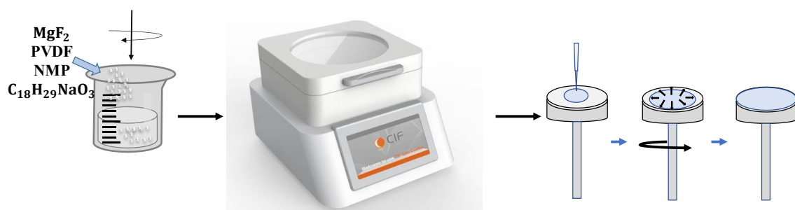
Figure 2. Process for the preparation of porous \text{MgF}_2 coatings.
