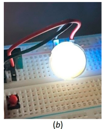
Figure 13. The appearance of the finished LED: three LEDs without phosphor coating (a) and an LED with a polymer lens containing phosphor in its composition (b).
