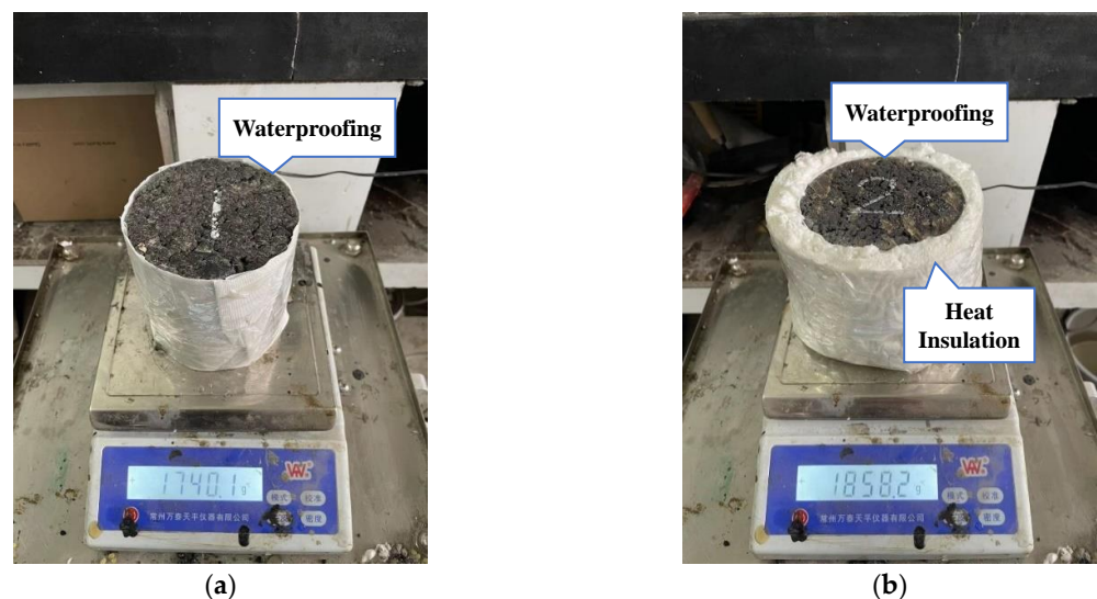
Figure 2. Simulation of curing schematic (a) waterproofing (b) heat insulation.
