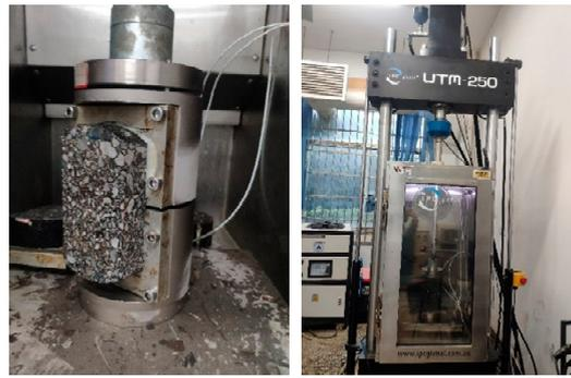
Figure 6. OT test setup.
