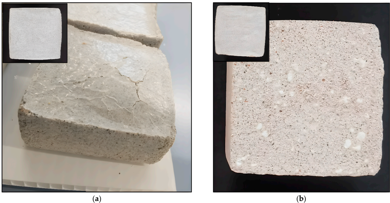
Figure 4. (a) MSD05 sample before (top left-hand corner) and after undergoing freeze–thaw cycles; (b) MSCD05 sample before (top left-hand corner) and after undergoing freeze–thaw cycles.
