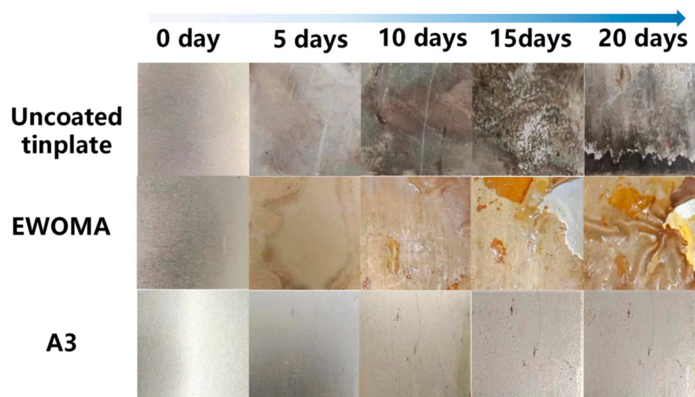
Figure 7. Optical photos with different surface corrosive results of uncoated tinplate, pure EWOMA and EWOMA-HEMA resin (A3 sample) coated on tinplate submerged in 5.0 wt% NaCl solution for different times.
