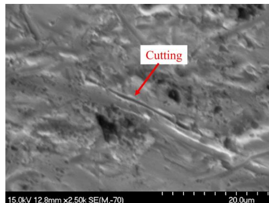
Figure 14. An example of a cutting deep groove on Ni-P-Tribaloy.
