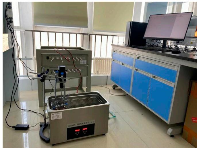
**Figure 1.** Photo of nanocomposite plating device.
