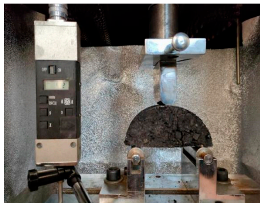
Figure 2. Semi-circular bending laboratory test.
